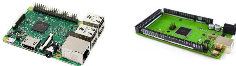
[1] RaspberryPi 3 Model B      [2] Arduino MEGA (compatible)
